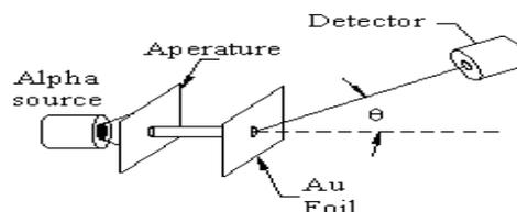
Figure 1. Scattering Geometry for  $\alpha$ -particles in the Rutherford Scattering
