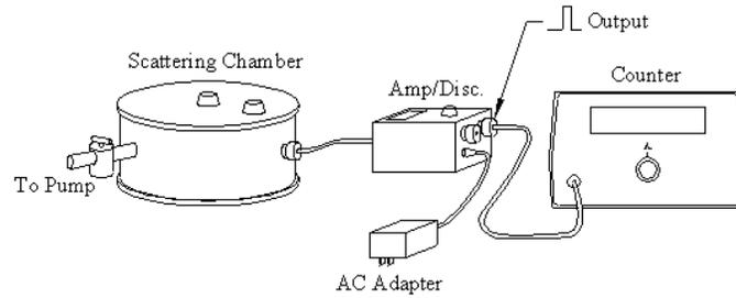
Figure 2. Experiment setup and electrical connections for Rutherford Scattering that includes a scattering chamber with shut off valve, pump(not shown), discriminator/preamplifier, AC adapter, and counter
