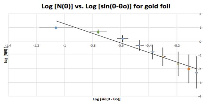
Figure 3. The plot of the data taken for  $\log[N(\theta)]$  against  $\log[\sin(\theta-\theta_0)]$  to determine if the line fit the Rutherford scattering equation
